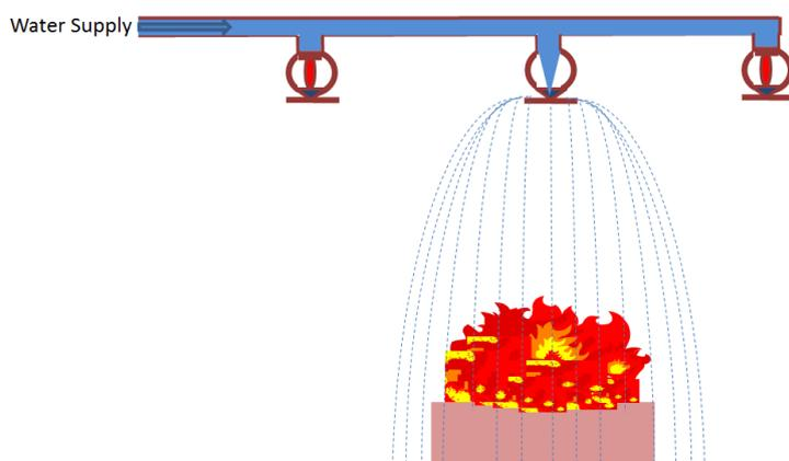
Sprinkler systems operate one sprinkler head at a time, directly over a fire
